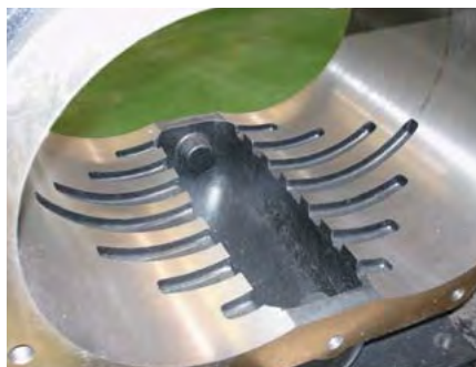
Pulse Eraser (pressure pulsation reduction mechanism)
